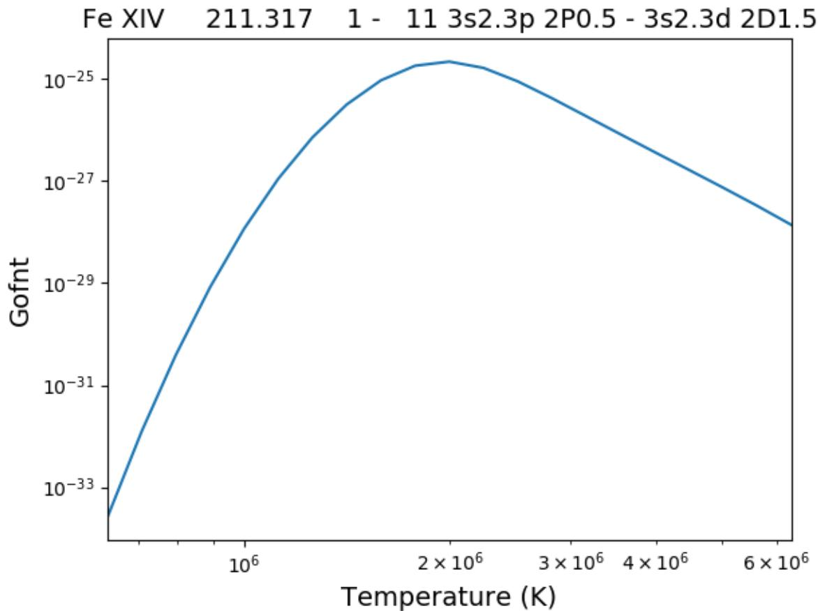
The G(n,T) calculation is stored in the Gofnt dictionary, with keys = ['gofnt', 'temperature', 'density']
