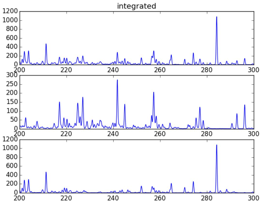
The integrated spectrum is formed by summing the spectra for all temperatures.
